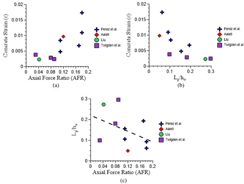
Figure 3. Experimental Result of Unbonded Post-Tensioned Walls at Drift Level of 2% (a) Concrete Strain vs Axial Force Ratio (AFR) (b) Concrete Strain vs  $L_p/h_w$  (c)  $L_p/h_w$  vs Axial Force Ratio (AFR)
